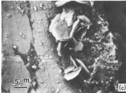
Figure 15 The surface of the steel fibre before being cast into the cement paste (a) and after being removed from the hardened paste (b), (c).
