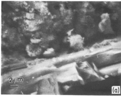
Figure 10 Higher magnification of the CH rim.
